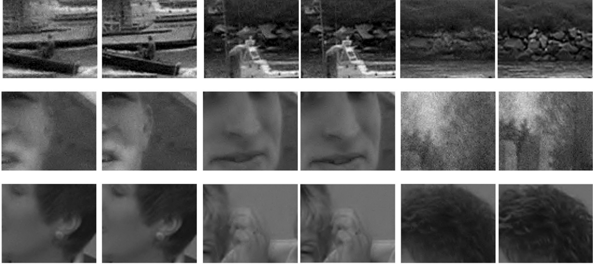
Fig. 6. Some reconstructed frames by DCVS (left) and DCVS-AM (right) at the same EMR: A side-by-side visual comparison
